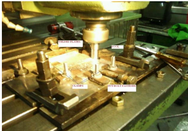
Fig. 1: Friction Stir Welding Setup
